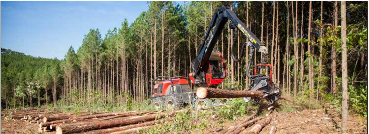
Pictured outside Vinton, Ohio, the Komatsu 931XC processes 200 tons of plantation pine per day. Crawford lists “the turning and self-levelling cab, fabulous stability, excellent traction and phenomenal fuel economy” as favorite features.
