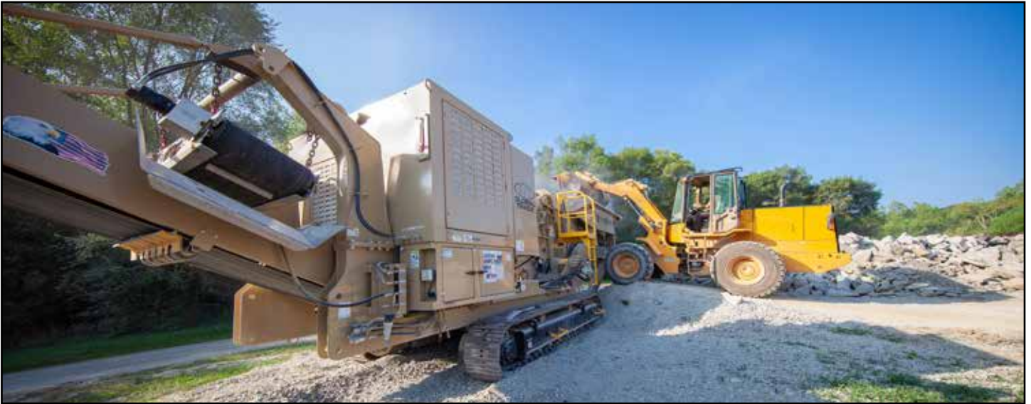
Operator Randy Bowman—a 36-year veteran—loads concrete into a GT440 producing 411/304 sand, as well as 57 and 2 products.
