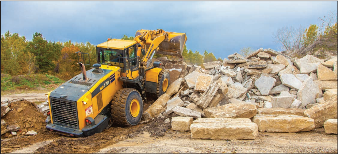
Arms Sand & Gravel Foreman Dan Mahne has been with the company over 20 years, and resolutely describes the Komatsu WA470 wheel loader as the quarry “workhorse.” The reliable machine is used for loading a variety of aggregate product, as well as processing incoming debris (above) in Newbury, Ohio.
